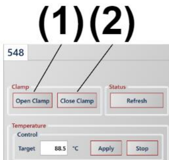
Figure 2: Operation of the “Active Clamping” mechanism with buttons for opening (1) and closing (2).
