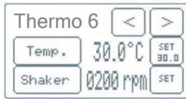
Illustration 24: Activate heating / cooling by touching the button Temp, which then appears black
